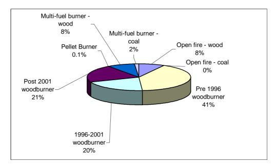
Figure 4-5: Relative contribution of different heating methods to average daily  $PM_{10}$  (July) from domestic heating in Turangi
