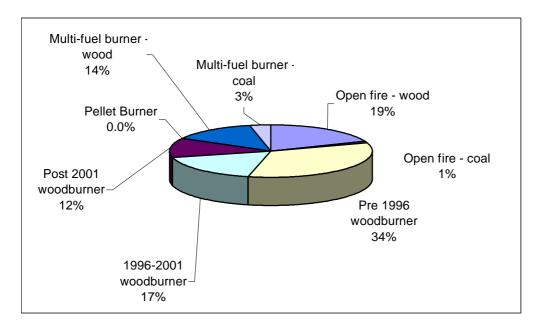
Figure 4-1: Relative contribution of different heating methods to average daily  $PM_{10}$  (July) from domestic heating in Te Awamutu
