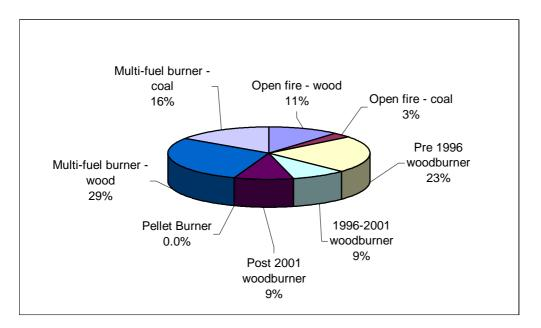
Figure 4-9: Relative contribution of different heating methods to average daily PM<sub>10</sub> (July) from domestic heating in Ngaruawahia
