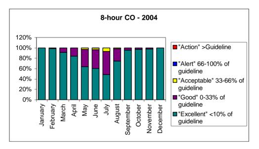
Figure 2-7: Comparison of 8-hour average CO concentrations measured in Hamilton during 2004 to MfE air quality indicator categories
