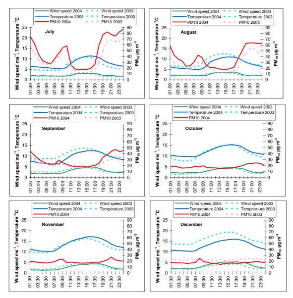
Figure 3-13: Hourly average PM10, wind speed and temperature values for 2003 and 2004 for each month from July to December
