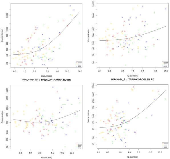
Figure E-1: Rating curves for the water quality monitoring sites with paired measured flow records. Continured
