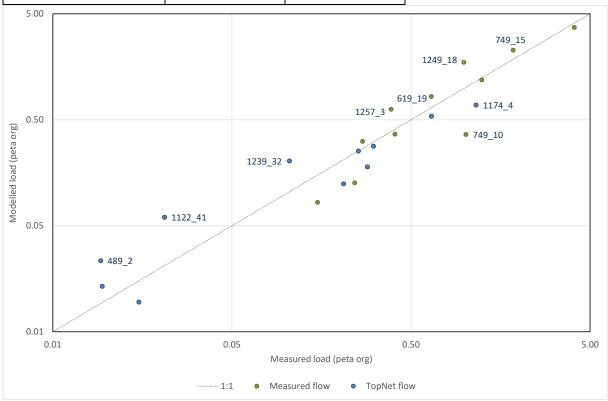
Figure 4-1: Comparison of modelled and measured load plotted on log scale Labels show load outliers discussed in the text.
