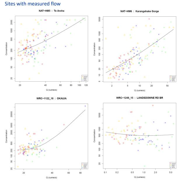
Figure E-1: Rating curves for the water quality monitoring sites with paired measured flow records.
