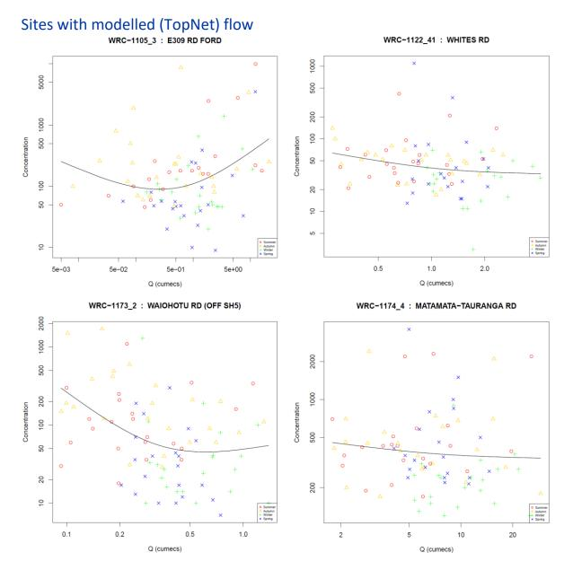
Figure E-2: Rating curves for the water quality monitoring sites with modelled (TopNet) flow records.
