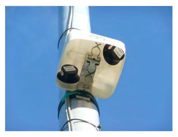
Figure 12.1: Duplicate radon detection badges co-located at an FH62 BAM monitoring site.
