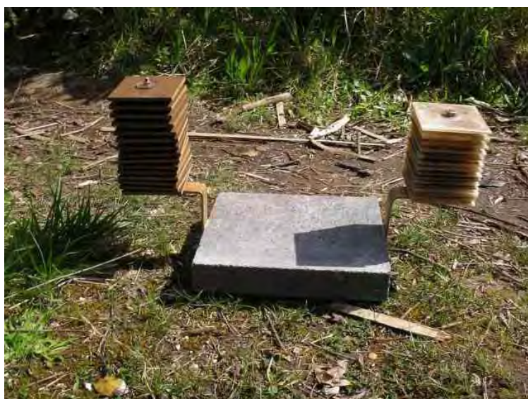
Plate 1: Paired multiplate samplers constructed from hardboard (left) and perspex (right) showing position of samplers in relation to the concrete paver.
