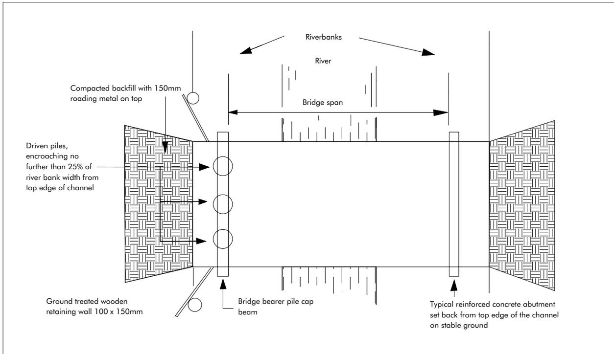
**Figure 32: Bridge plan view**
