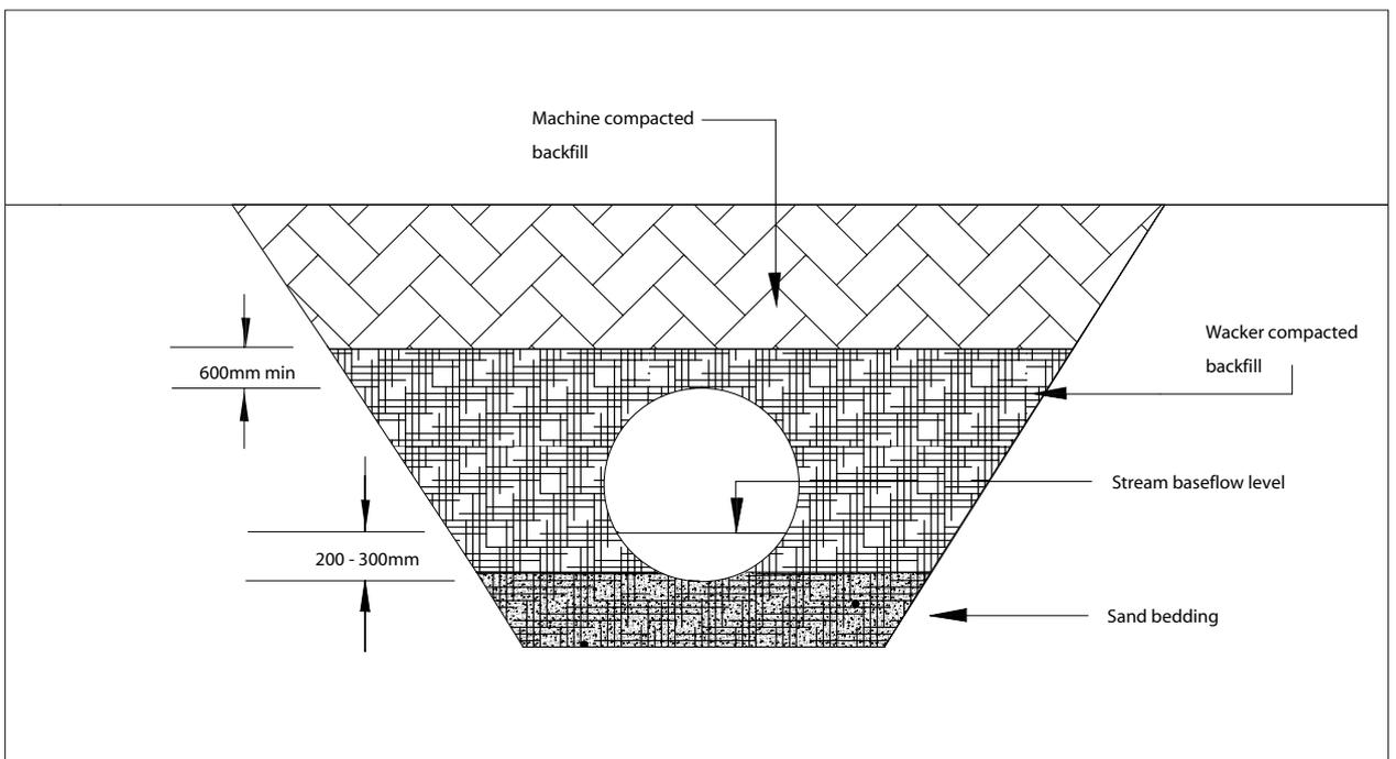
**Figure 36: Culvert crossing outlet**
