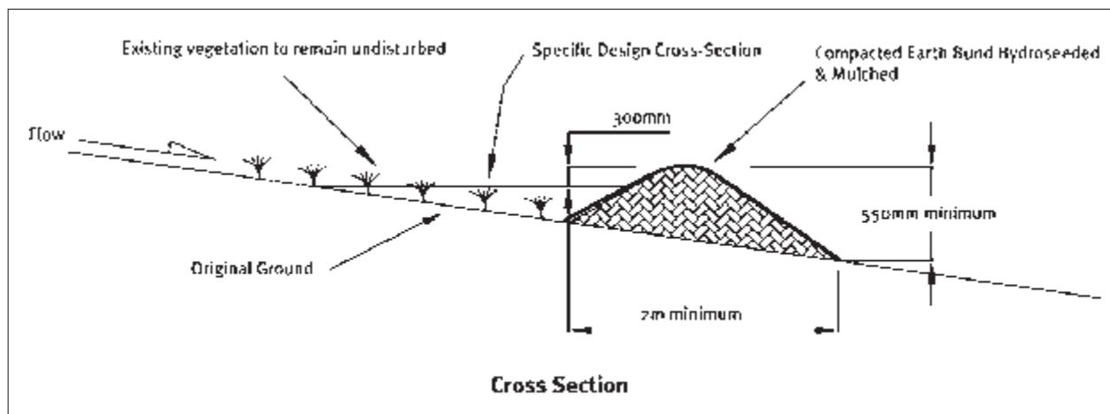
**Figure 2: Clean Water Diversion Channel**
