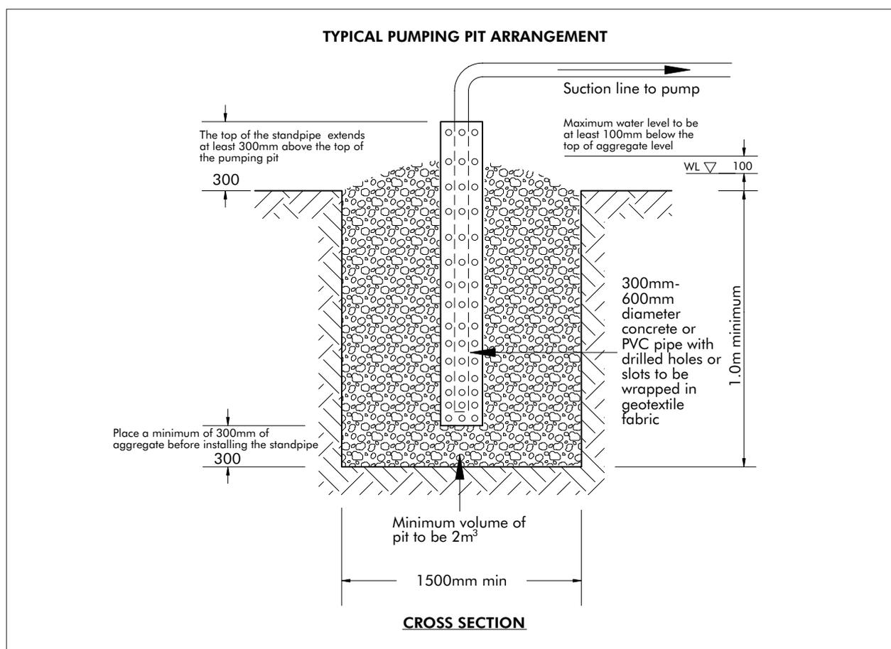
**Figure 29: Sump/sediment pit**
