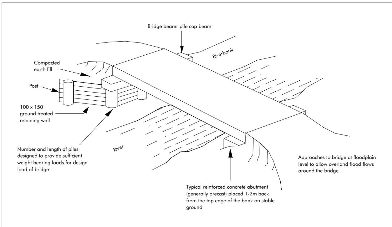
**Figure 33: Small bridge installation**
