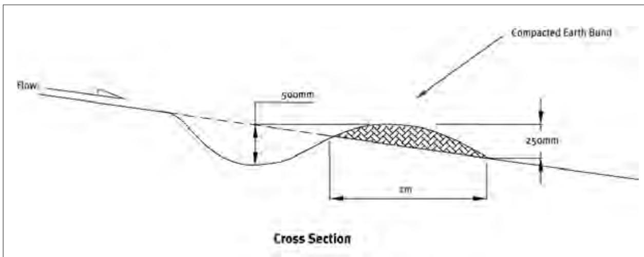
**Figure 4: Contour Drain**
