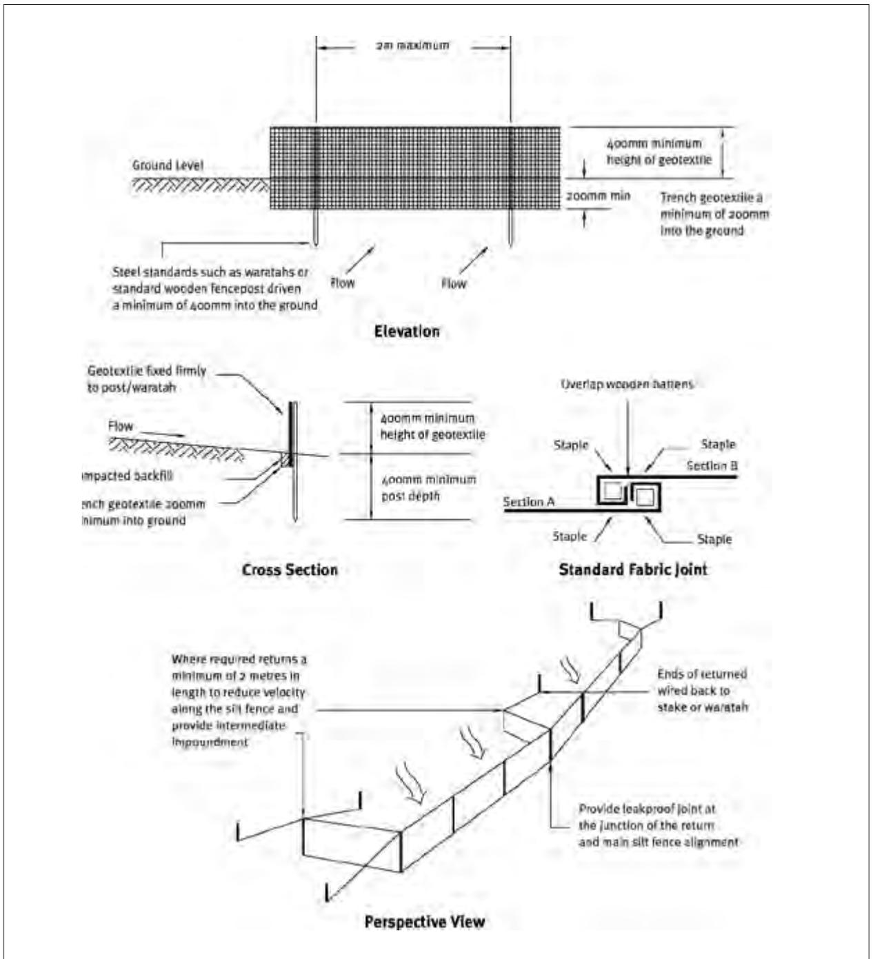
**Figure 24: Silt fence**
