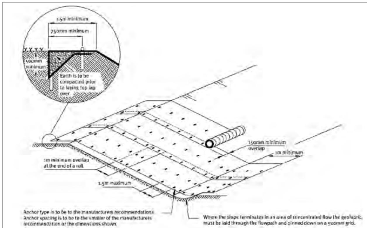
**Figure 11: Geotextile Laid on Slope**
