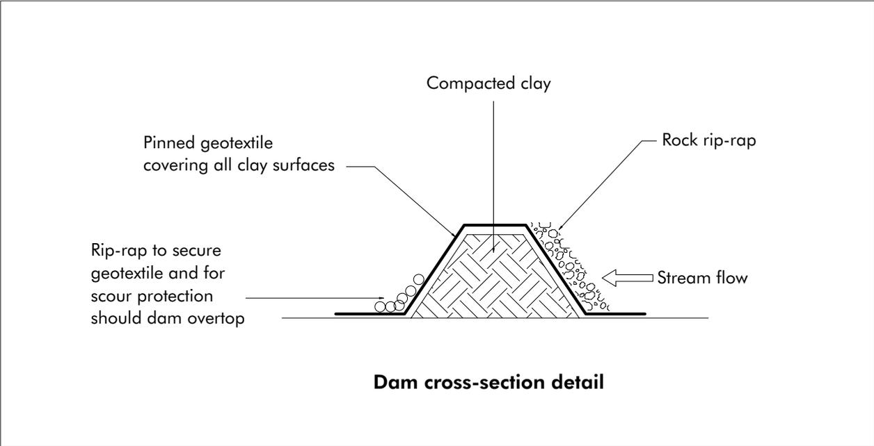
**Figure 31: Temporary watercourse diversion dam detail**
