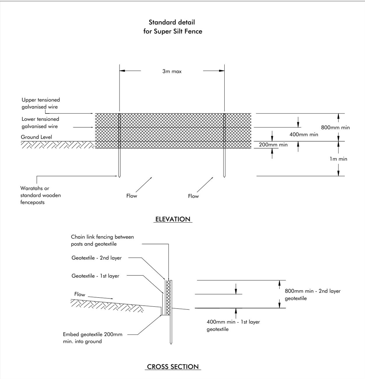
**Figure 25: Super silt fence**
