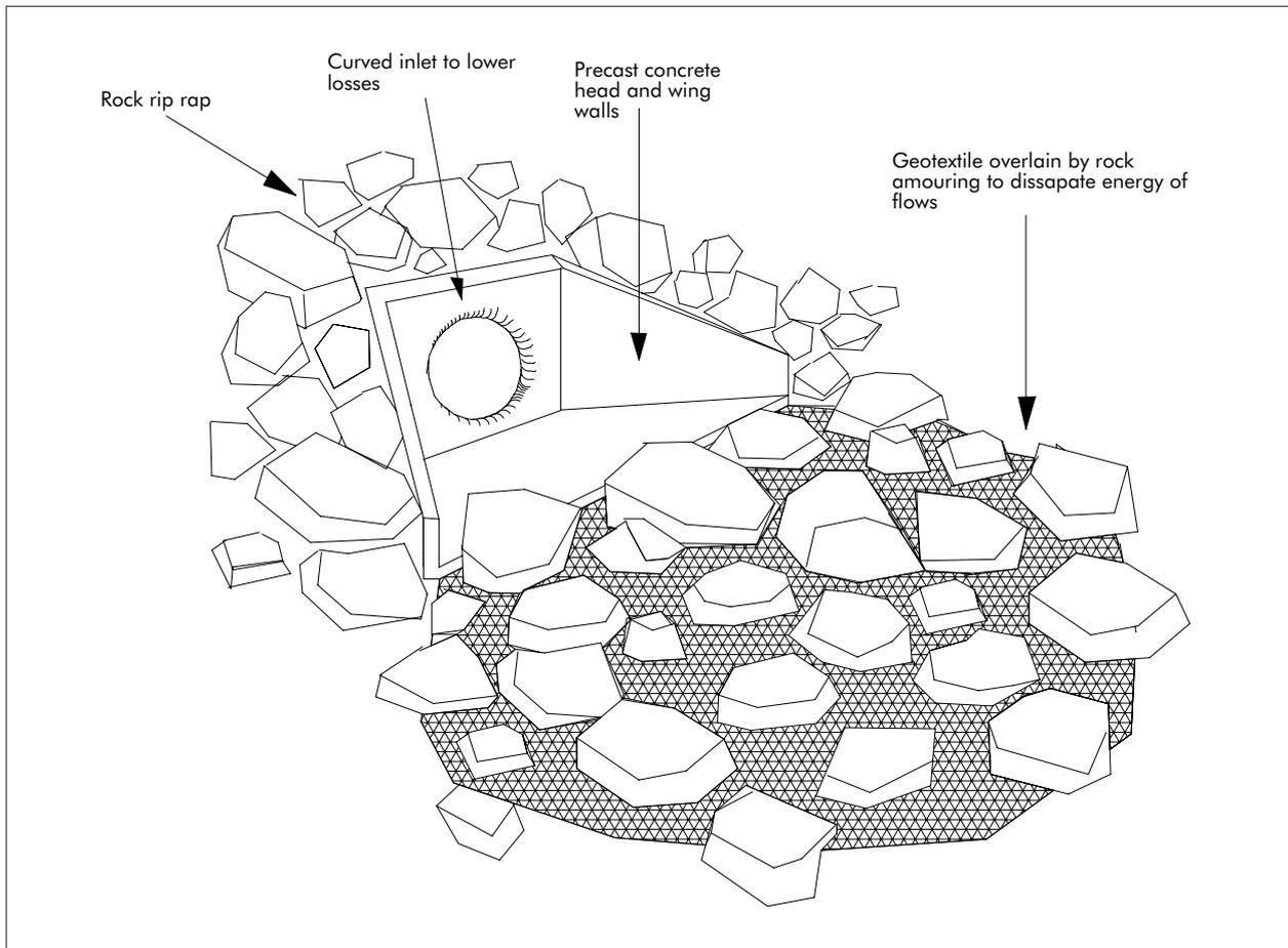
**Figure 34: Culvert inlet using precast headwall**
