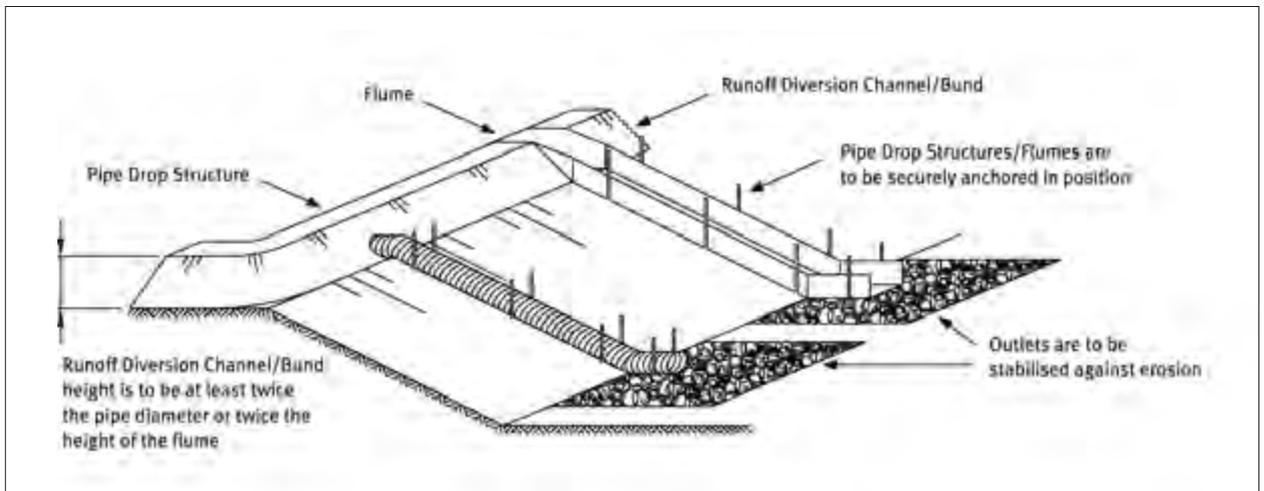
**Figure 14: Pipe/flume drop structures**
