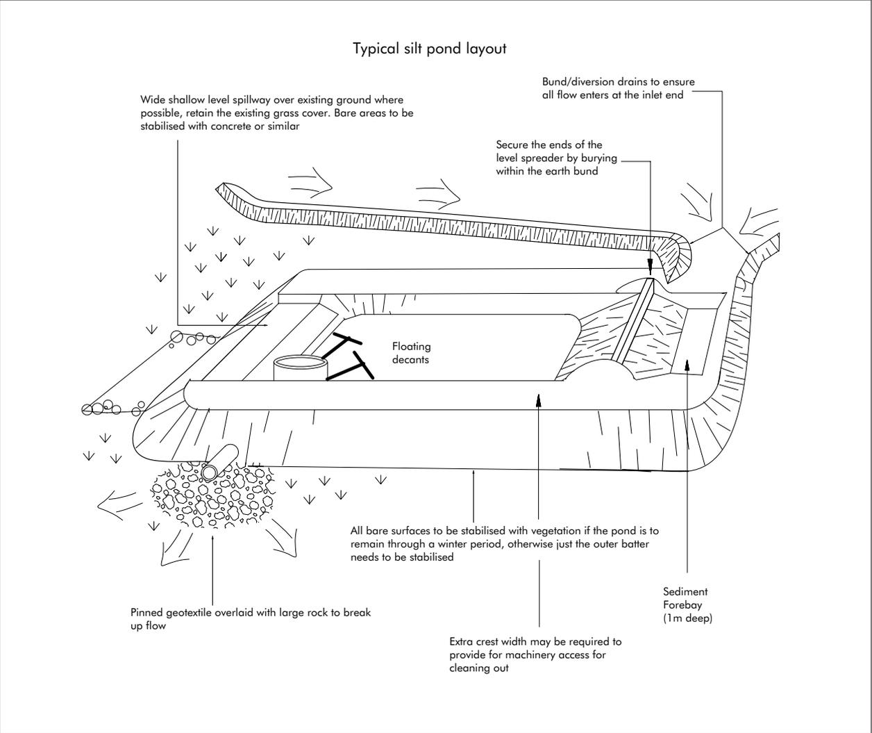
**Figure 23: Sediment retention pond**
