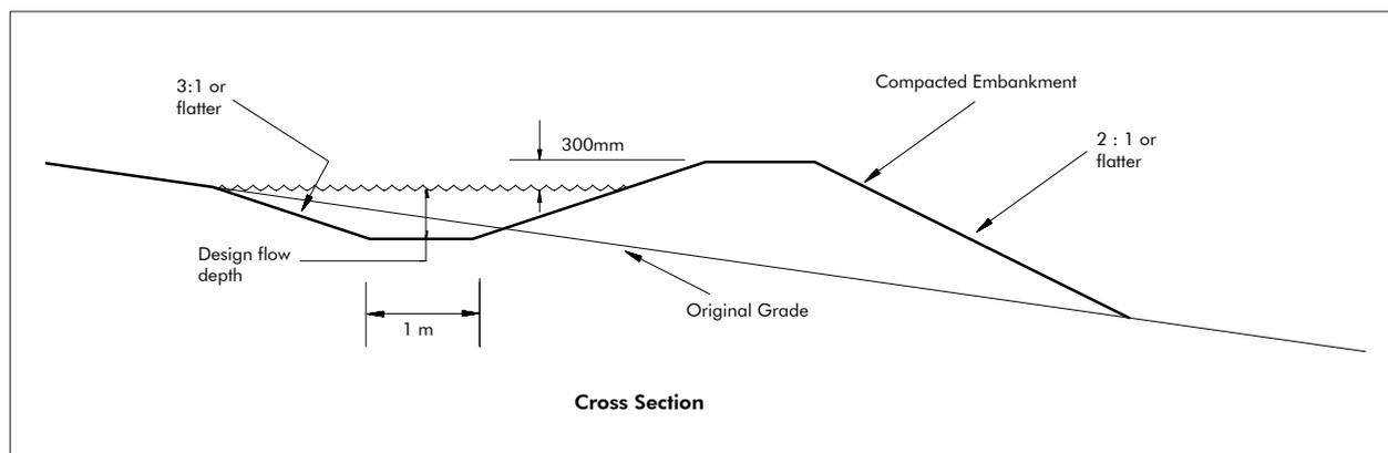
**Figure 3: Runoff Diversion Channel**
