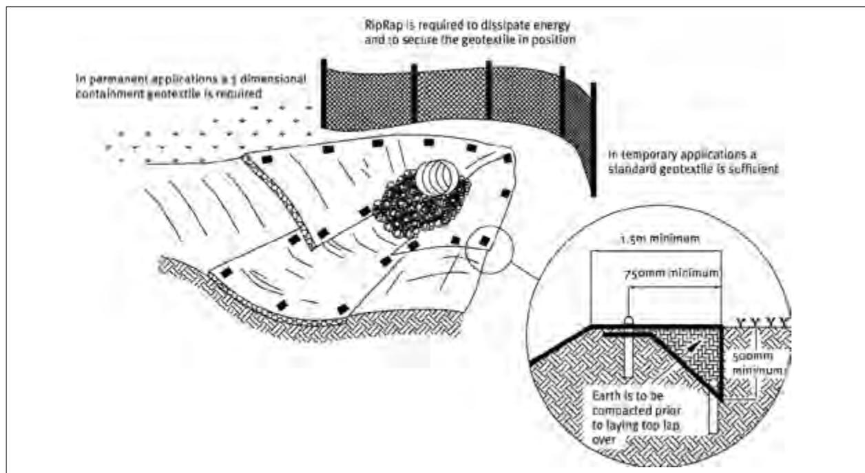
**Figure 12: Geotextile at Culvert Outlet**
