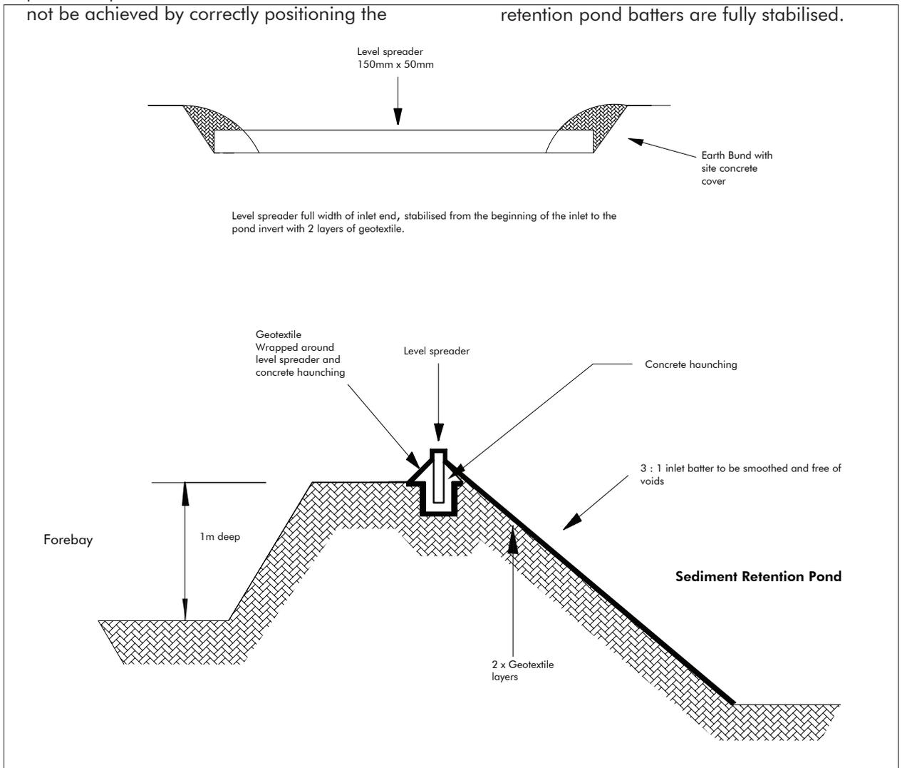
**Figure 18: Pond level spreader**
