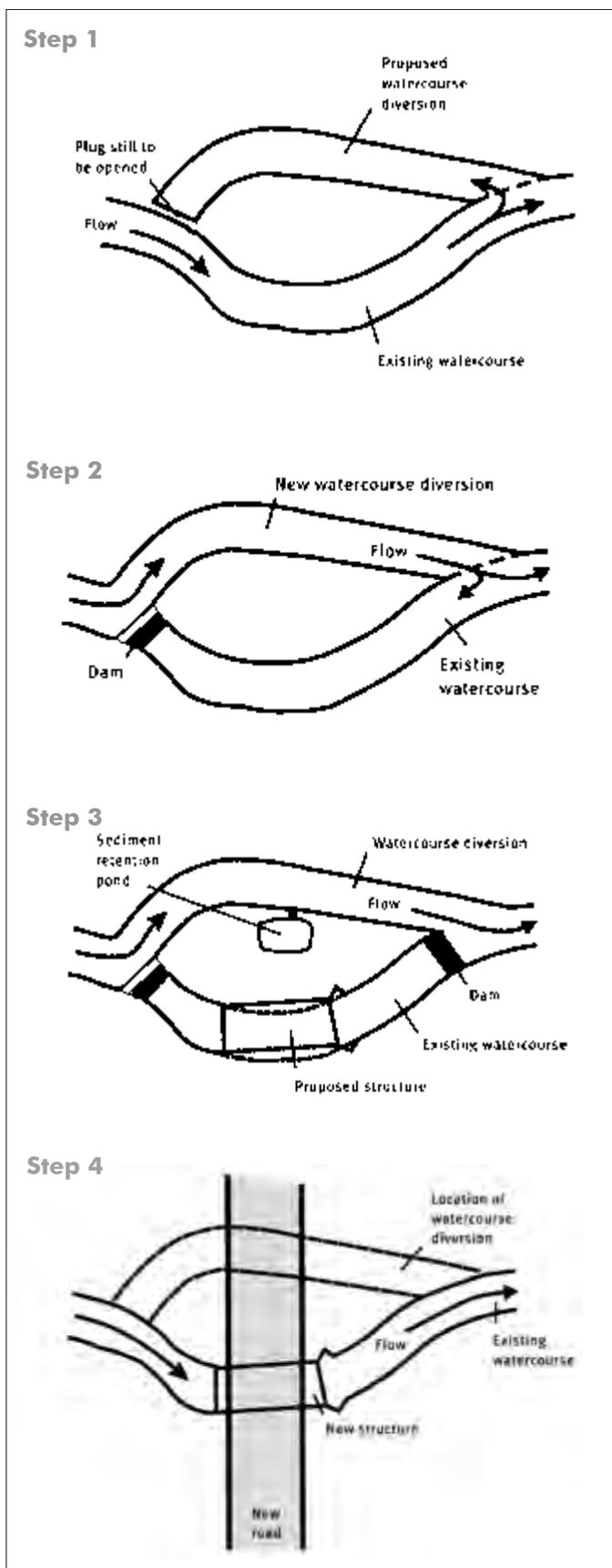
**Figure 30: Temporary watercourse diversion works sequence**
