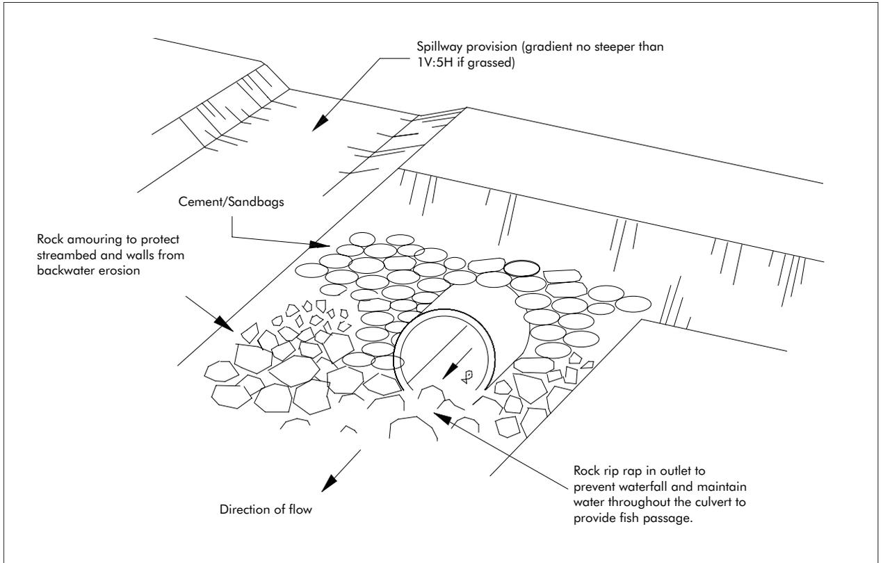
**Figure 35: Culvert outlet protection**
