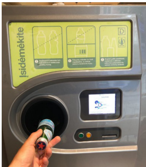
An RVM in Lithuania - the two icons stacked on top of each other in the top right hand side of the machine's instructions show that both single-use (top icon) and reusable bottles (bottom icon) are accepted. Image by sensoneo.com
