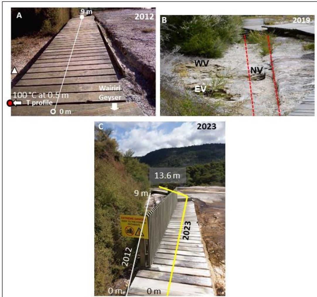
Figure 20: Sites G9 (2012) and SW15 (2023). (A) Overview of the 2012 site G9. (B) The new vents in 2019 and the new boardwalk. (C) Relationship between 2012 and 2023 GPR profiles shown.
