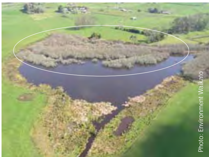
The wetland margins of Lake Komakorau are being extensively restored: all willow (circled) has been removed, silt traps constructed and a planting programme using natives developed.
