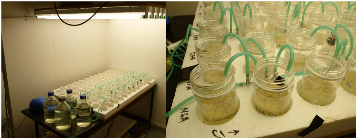
Figure 2: Bioassay incubations in a controlled temperature room under artificial lighting. (Left) showing the arrangement of the 48 nutrient addition incubation jars (green aeration tubes) beside the 48 non-aerated zooplankton dilution incubation jars (no tubes). (Right) a close-up of the aeration bubblers in the nutrient addition incubation jars. Large bottles are incubations of big zooplankton.
