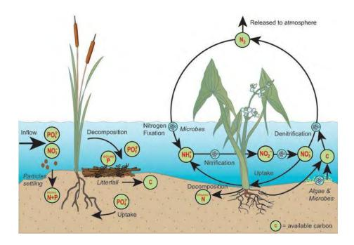
**Figure 8**. Simplified conceptual diagram of the nitrogen and phosphorus cycle in wetlands. Source: Wetlands Initiative
