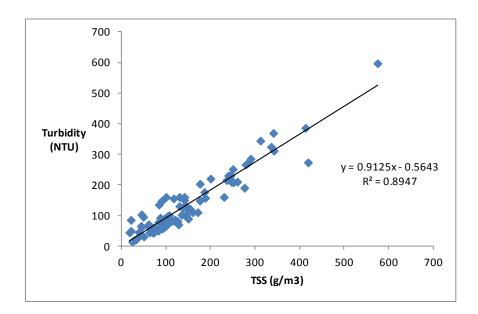
**Figure 15**. Relationship between Total Suspended Solids (g/m3) and Turbidity (NTU) from the Pungarehu Canal monitoring site. Source: WRC monitoring data 1995-2013.
