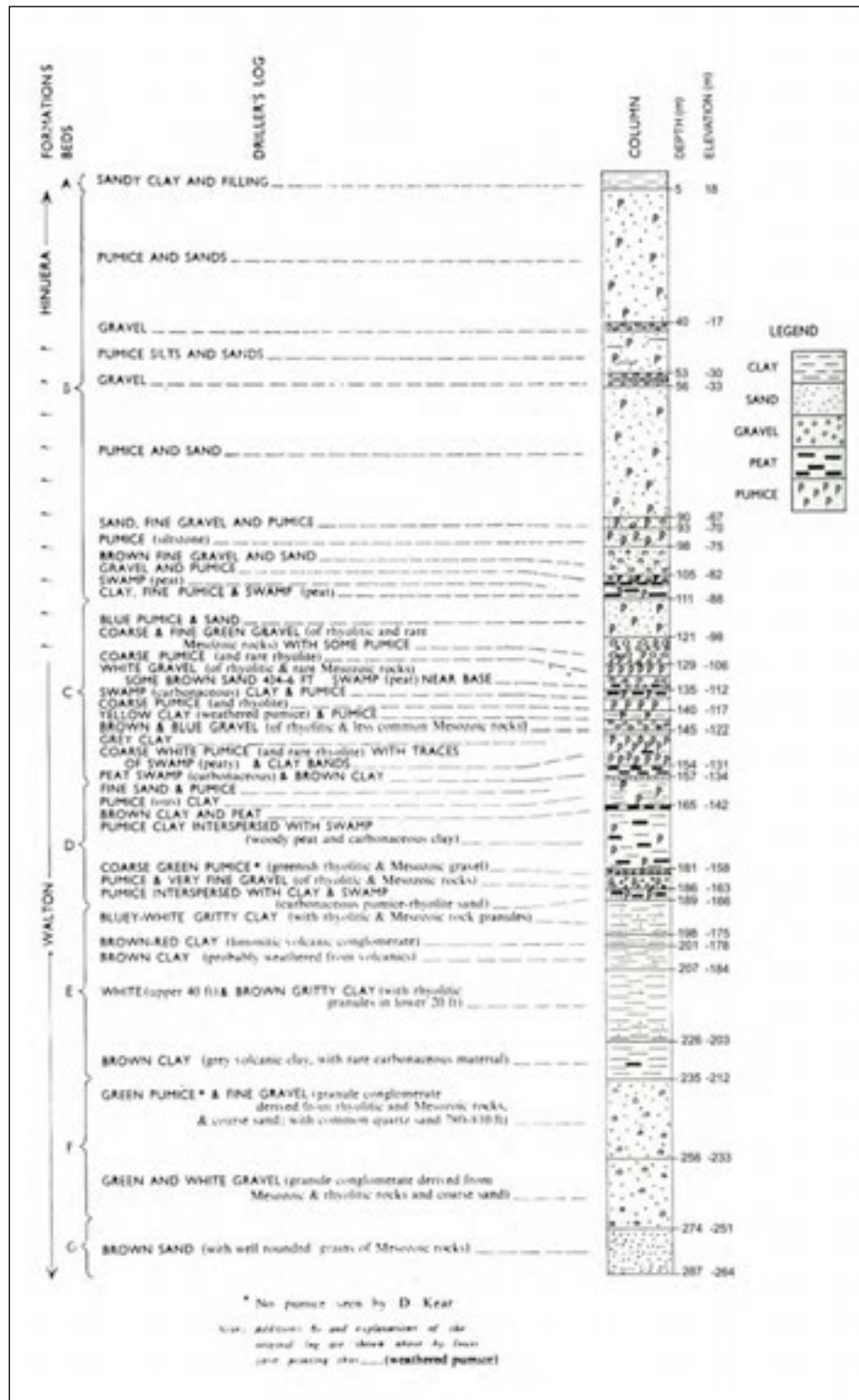
Figure 2.11 Lithological log of the approximately 287 m deep drill hole near Morrinsville (Kear and Tolley 1957).
