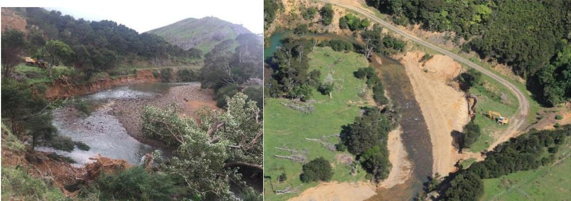
**Figure 12: Damage on the Waikawau River, and (right) temporary bund in place to prevent erosion of hillside at the same location**
