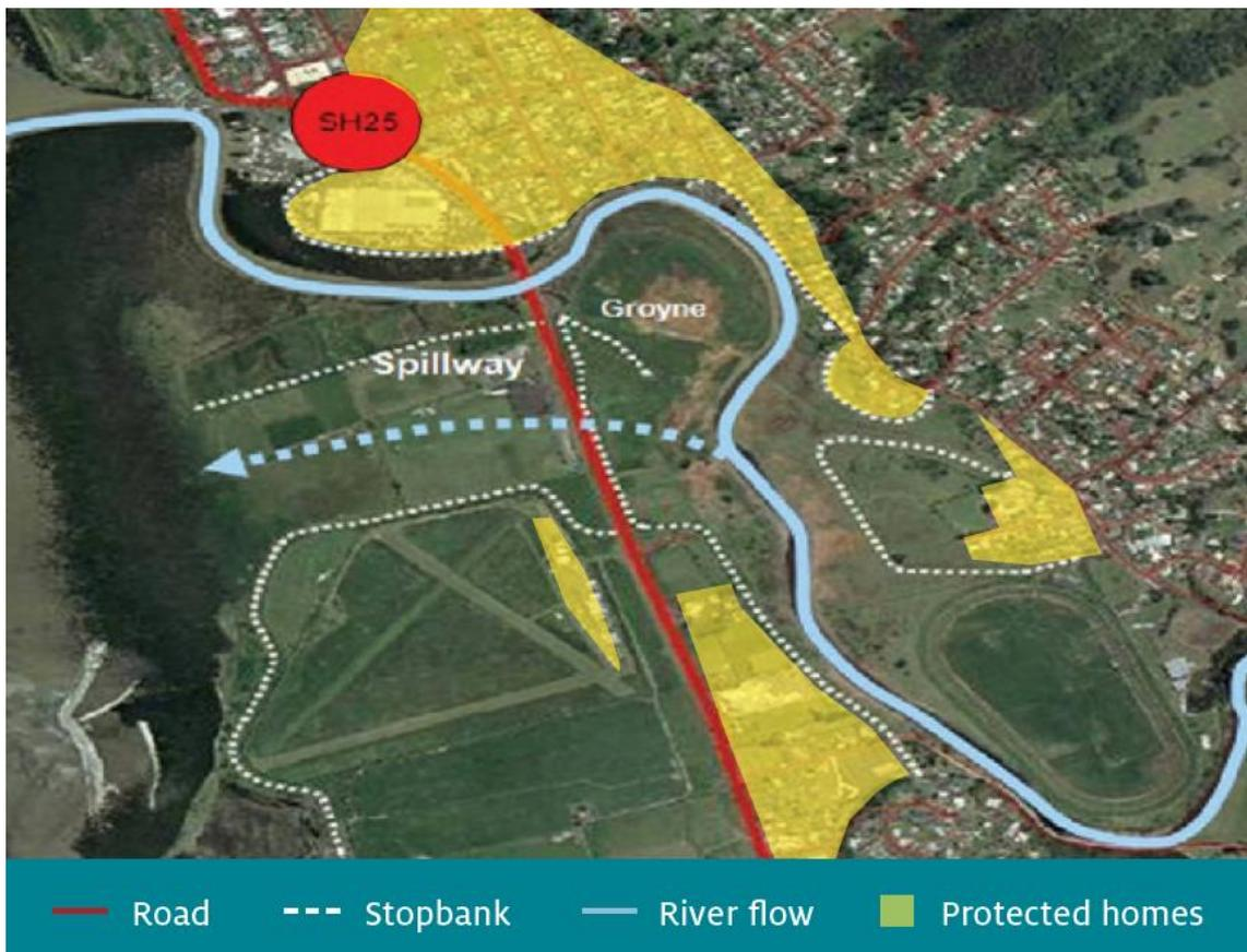
Figure 6: Diagram showing the Kauaeranga River flood protection infrastructure and spillway at the southern end of Thames.
