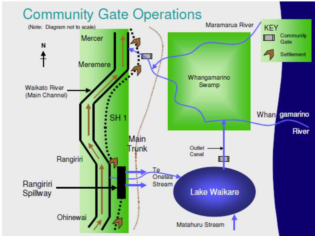
Figure 8: Conceptual diagram of the Lower Waikato Control Scheme.
