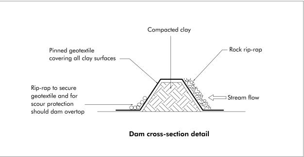
Figure 31: Temporary watercourse diversion dam detail
