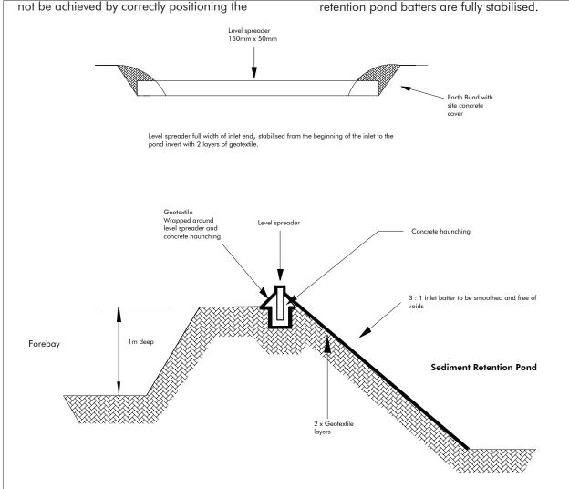
Figure 18: Pond level spreader
