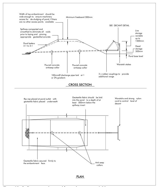
Figure 19: Sediment retention pond for catchments up to 1.5 ha
