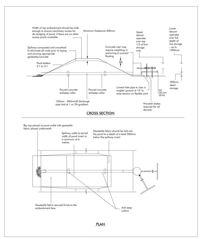
Figure 20: Sediment retention pond for catchments between 1.5 And 3 ha
