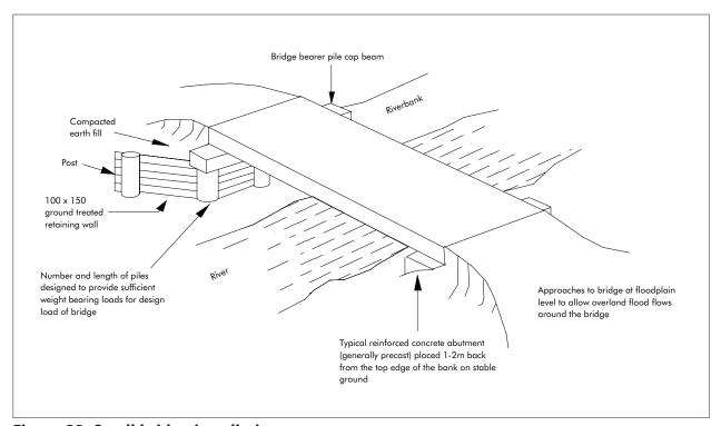
Figure 33: Small bridge installation
