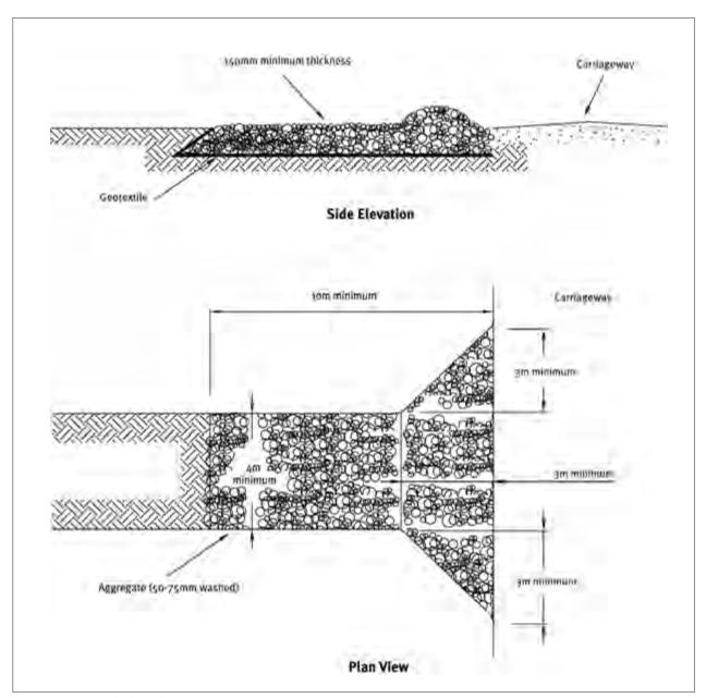
Figure 13: Stabilised construction entrance
