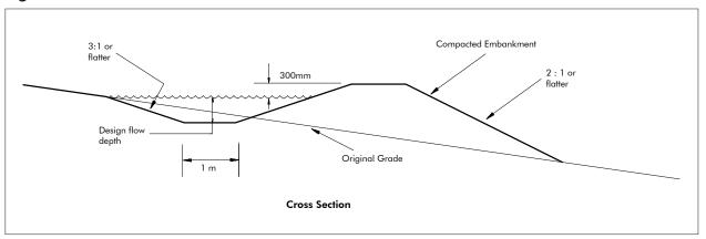
Figure 3: Runoff Diversion Channel
