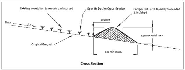
Figure 2: Clean Water Diversion Channel
