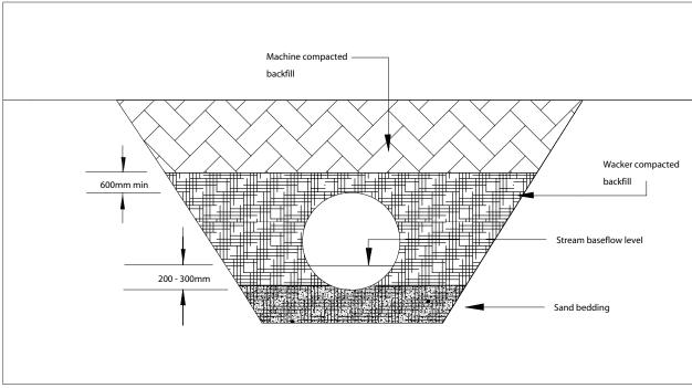
Figure 36: Culvert crossing outlet
