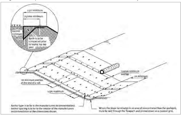
Figure 11: Geotextile Laid on Slope
