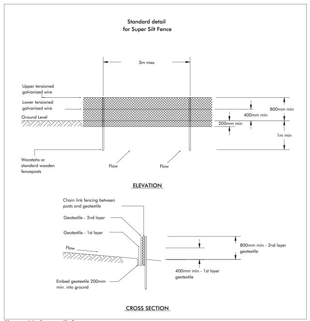
Figure 25: Super silt fence
