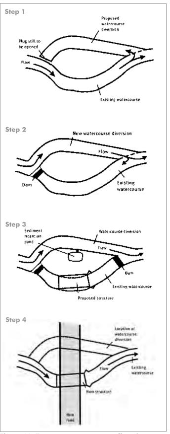
Figure 30: Temporary watercourse diversion works sequence
