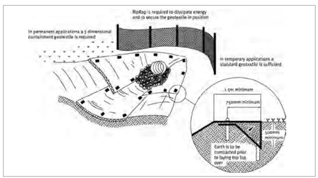
Figure 12: Geotextile at Culvert Outlet
