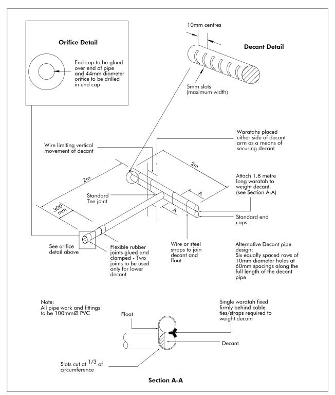
Figure 22: Sediment retention pond - decant detail
