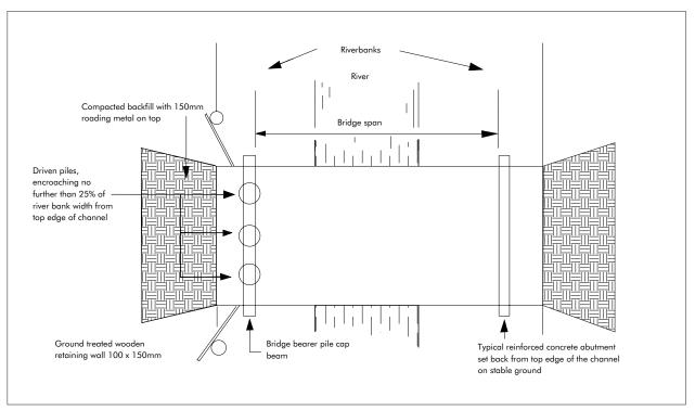
Figure 32: Bridge plan view
