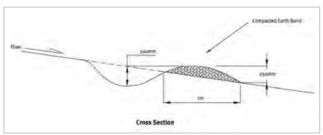
Figure 4: Contour Drain
