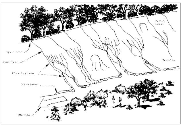
Figure 1: Types of erosion common in the Waikato region
