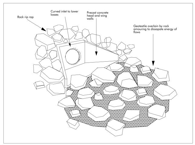
Figure 34: Culvert inlet using precast headwall
