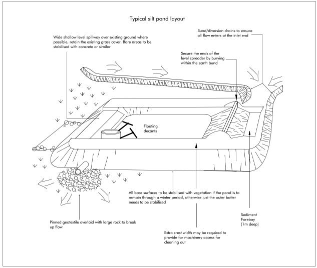
Figure 23: Sediment retention pond
