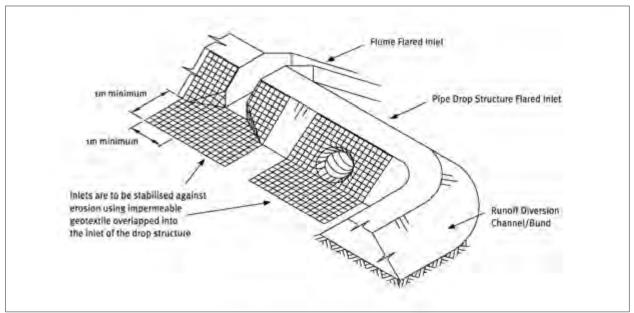
Figure 15: Flume design specifications (for catchments up to 0.5 ha)
