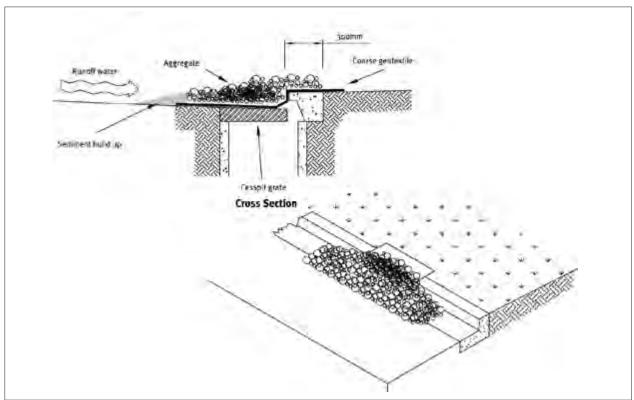
Figure 27: Stormwater inlet protection - filter media design
