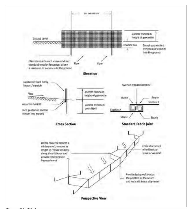
Figure 24: Silt fence
