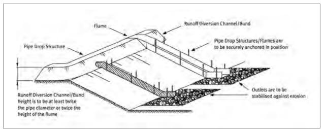
Figure 14: Pipe/flume drop structures
