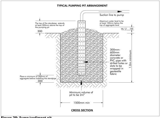
Figure 29: Sump/sediment pit
