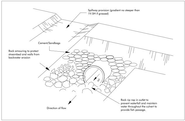
Figure 35: Culvert outlet protection
